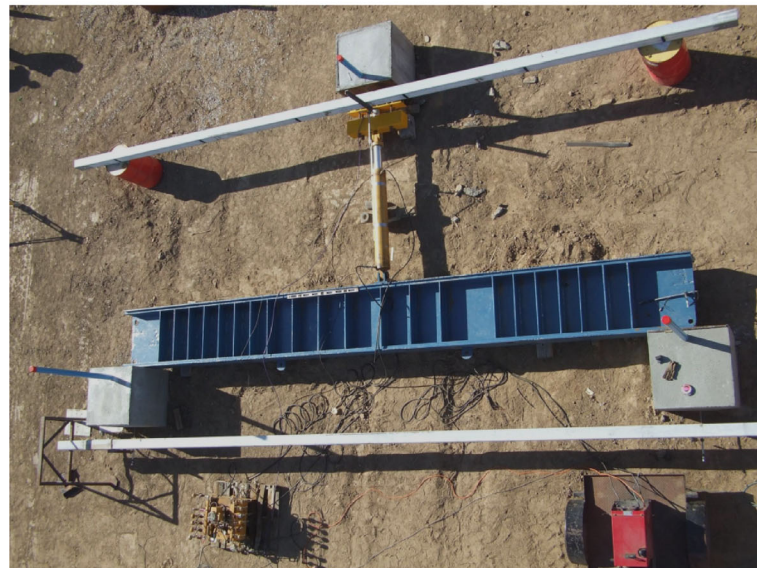
Fig. 3 Field test of a laterally loaded pile in a GRR wall. (a) Cross section; (b) Top view of setup for a single pile test
