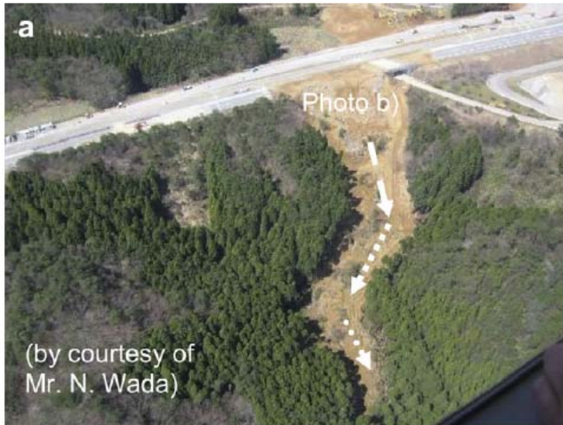
Failure of an embankment of Noto toll road (at site No. 32) caused by 2007 Noto-hanto earthquake.
