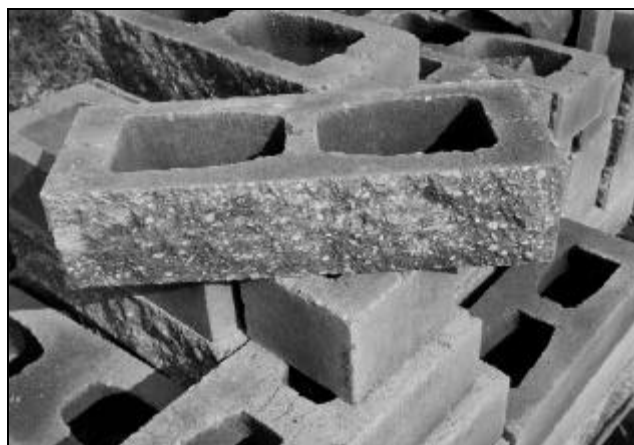
Photo 5. Half-High Split-Face Block at Minnesota Site
