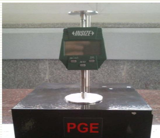
Thickness measurement apparatus
